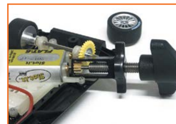
Pull the pinion leaving motor and crown in place
